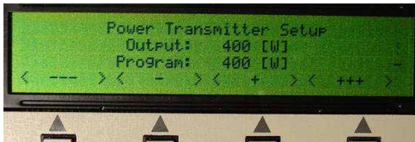
Fig.6.6: Power Setup Screen at the end, it must coincide with the external wattmeter reading
