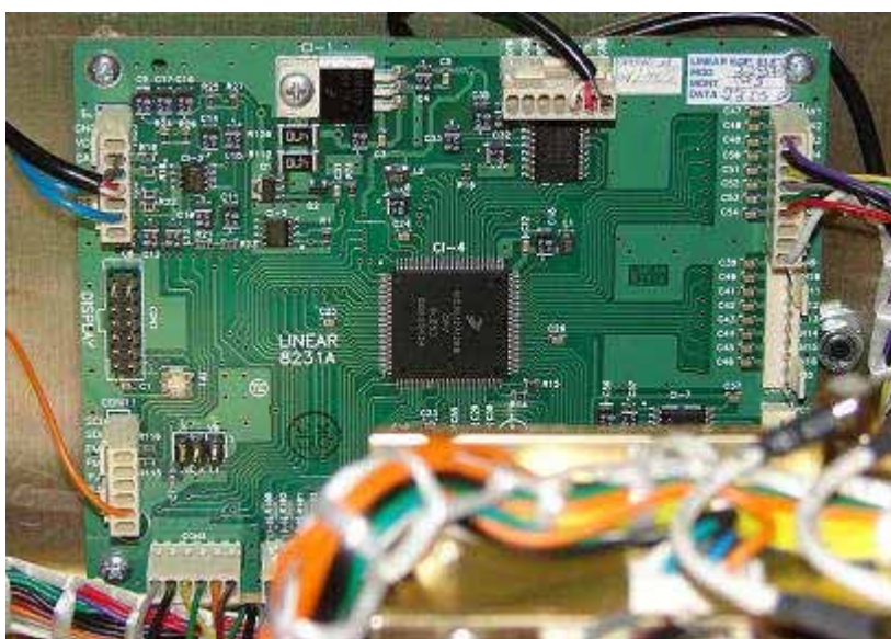
Fig.3.14: SCU assembled at the exciter drawer GV4456 – module 4456
