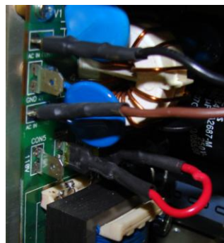
Fig.6.4: Jump connection for 110Vac operation, (CON4-CON3)
