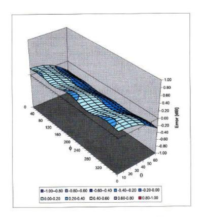
Spherical Isotropy Error < ± 0.4 dB
