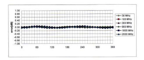
Axial Isotropy Error < ± 0.2 dB
