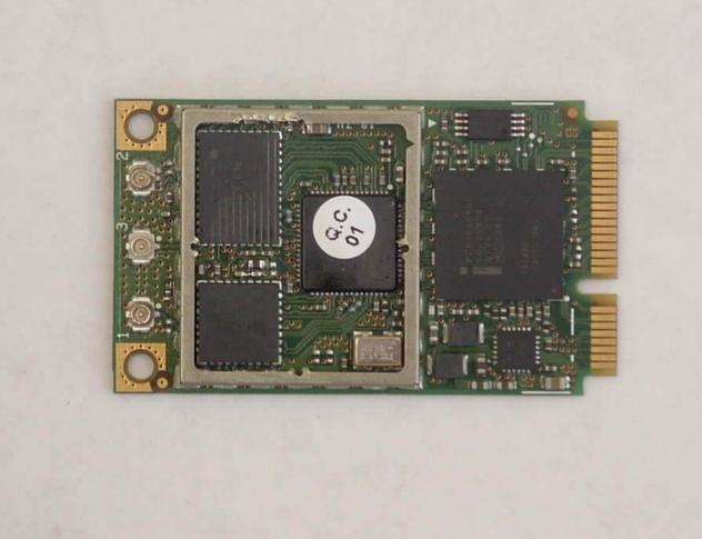
Top View "Shielding removed"
