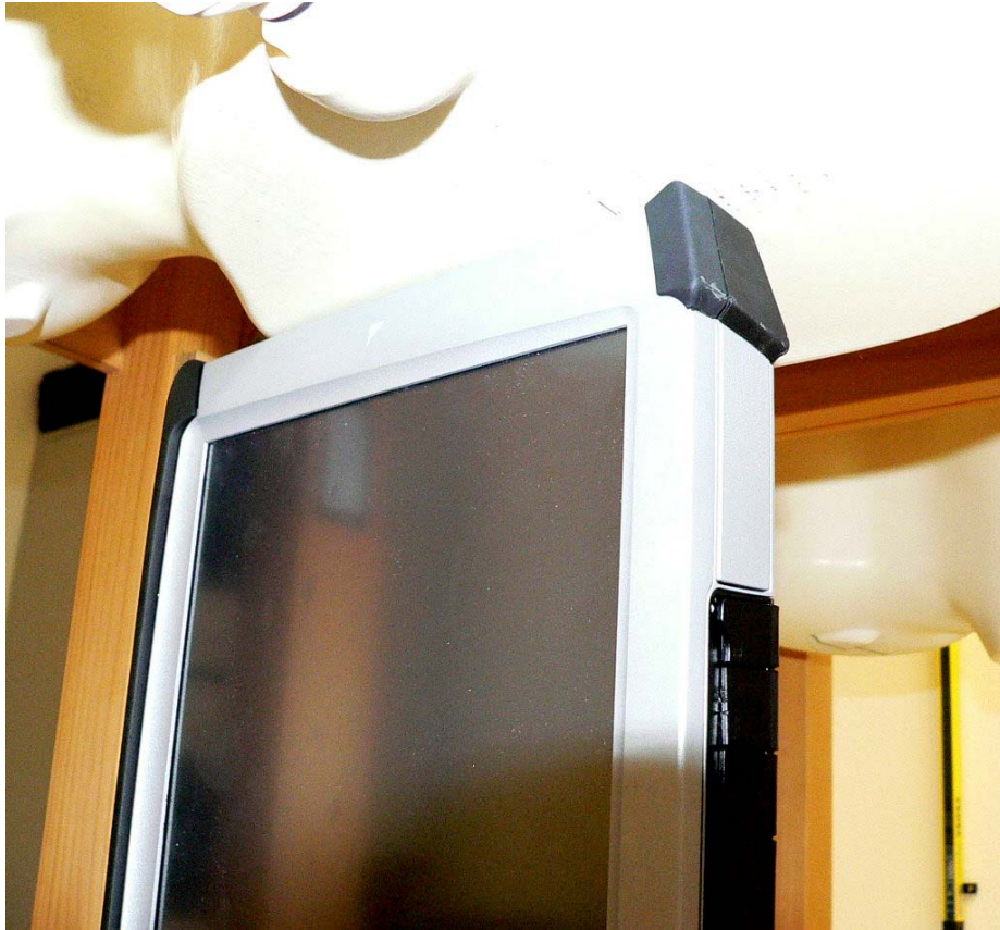
Fig. 31: Tested position for Bluetooth Antenna, side edge touching the phantom(front view)
