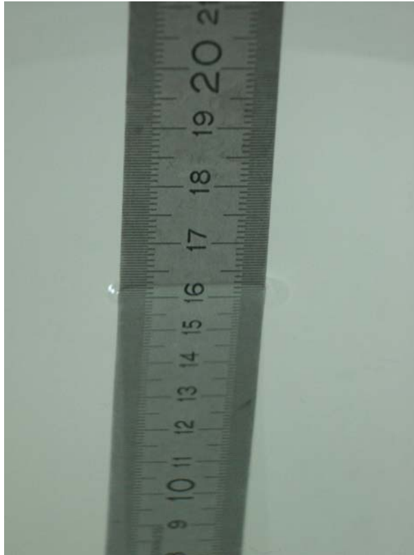
Fig. 33: Liquid depth for 2450 MHz Body measurements.
