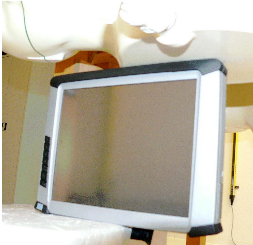
Fig. 27: Tested position for Antenna 2, upper edge touching the phantom (front view).
