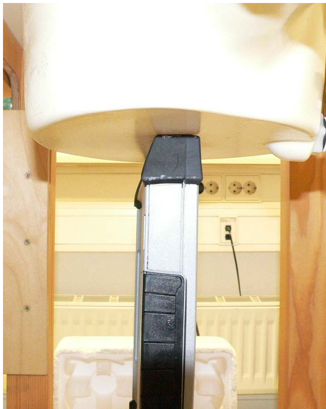
Fig. 30: Tested position for Antenna 3, side edge touching the phantom (side view).
