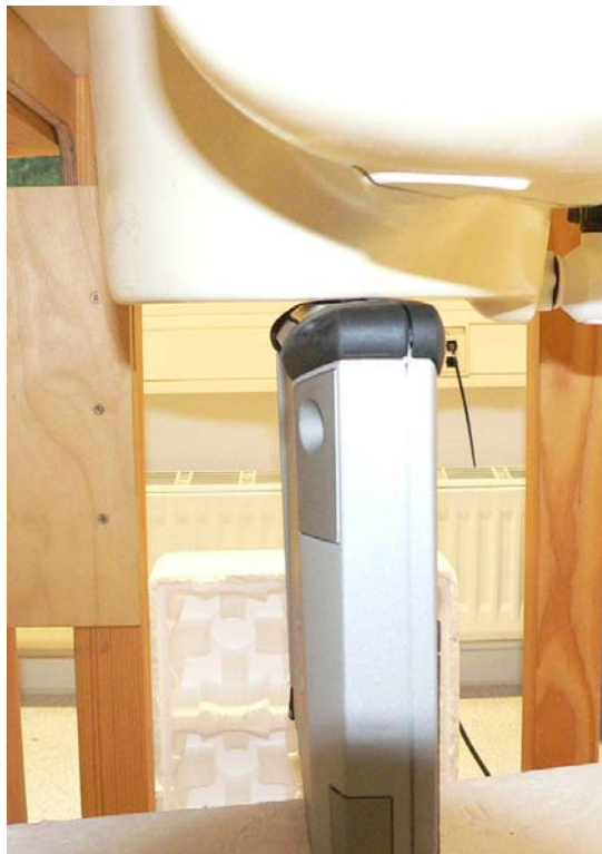
Fig. 28: Tested position for Antenna 2, upper edge touching the phantom (side view).
