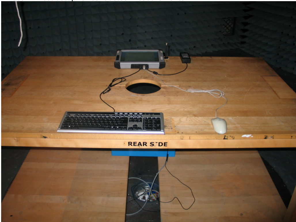
Photo 2: Test setup for radiated measurements
