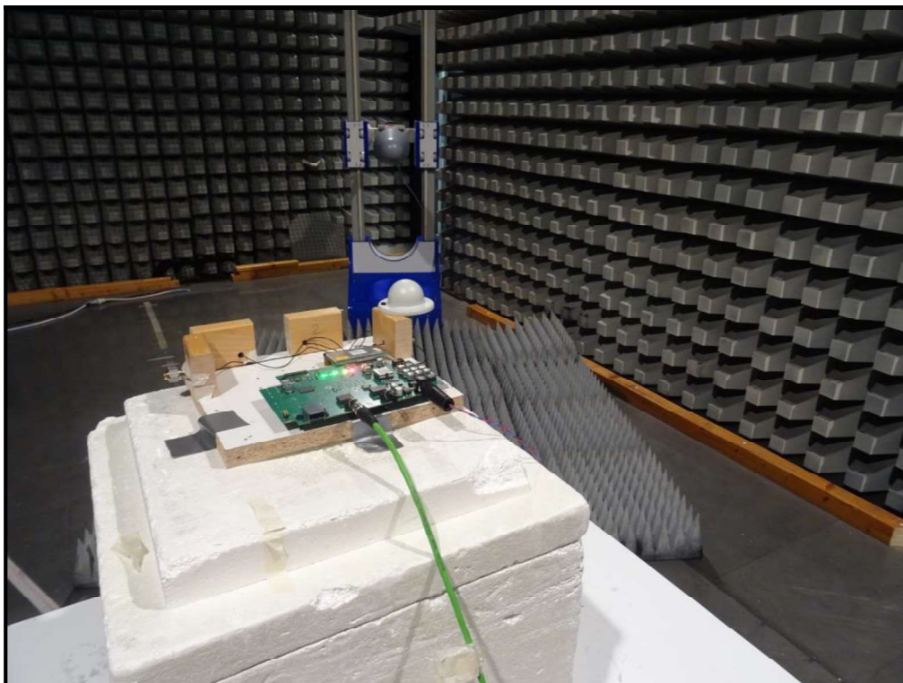
Photo 13:EUT- SISO PORT 1 (Ports 2,3 & 4 Terminatd with 50 \Omega )
