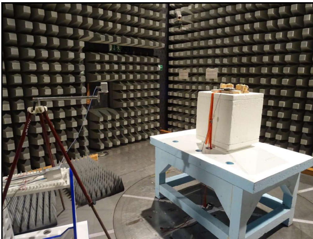
Photo 8: Terminated Ports 1+2+3+4 with 50 \Omega
