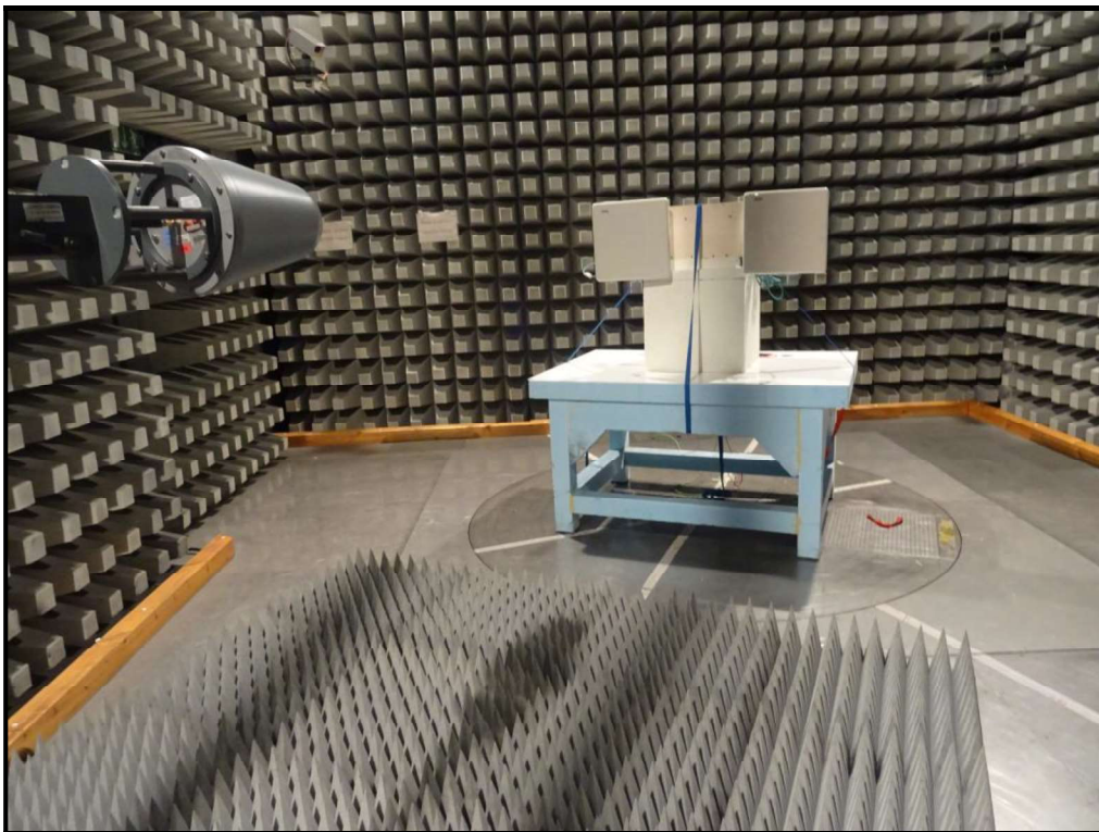
Photo 54:EUT- MIMO PORT 1+2+3 (Port 4 Terminatd with 50 \Omega )
