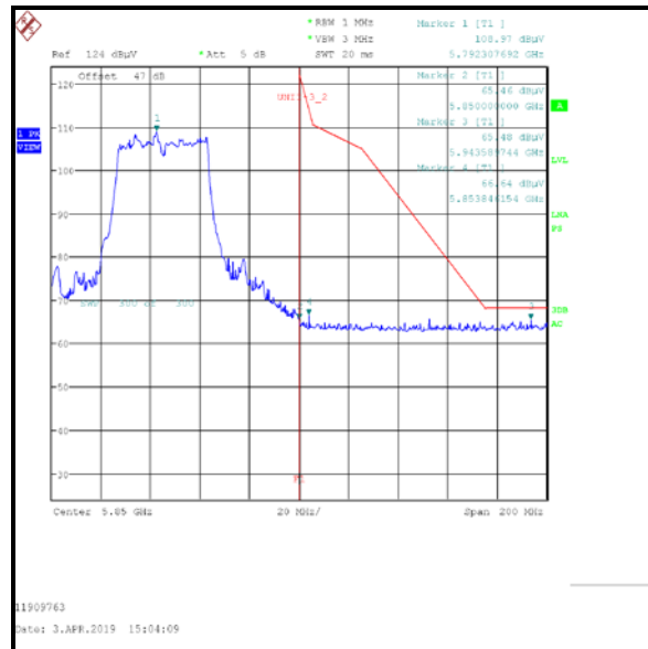
Upper Band Edge Measurement
