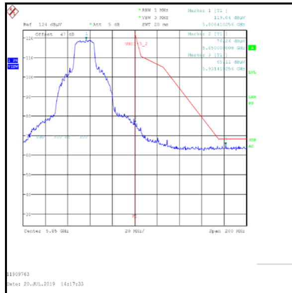
Upper Band Edge Measurement
