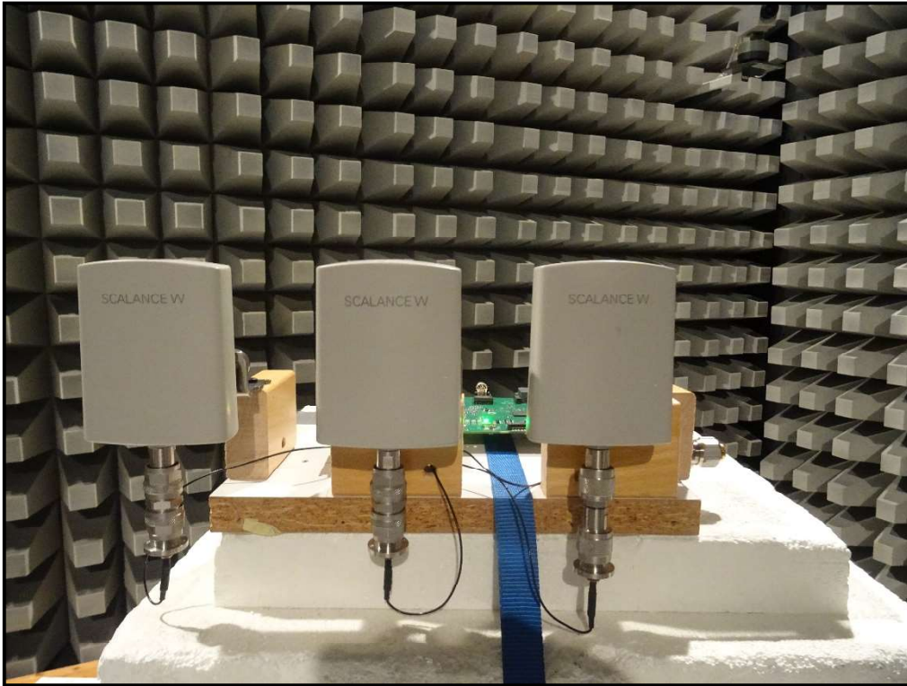
Photo 35: EUT- MIMO PORT 1+2+3 (Port 4 Terminated with 50 \Omega )
