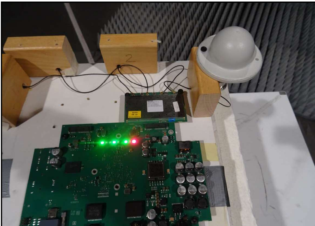
Photo 12: EUT- SISO PORT 1 (Ports 2,3 & 4 Terminated with 50 \Omega )
