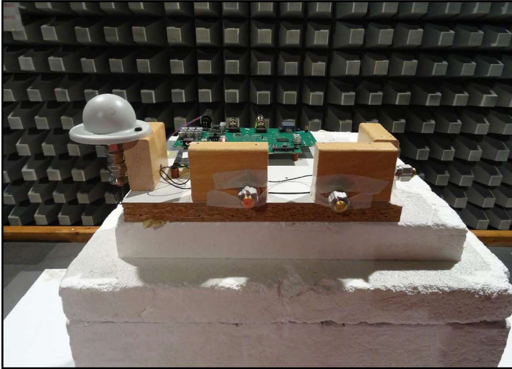
Photo 11: EUT- SISO PORT 1 (Ports 2,3 & 4 Terminated with 50 \Omega )
