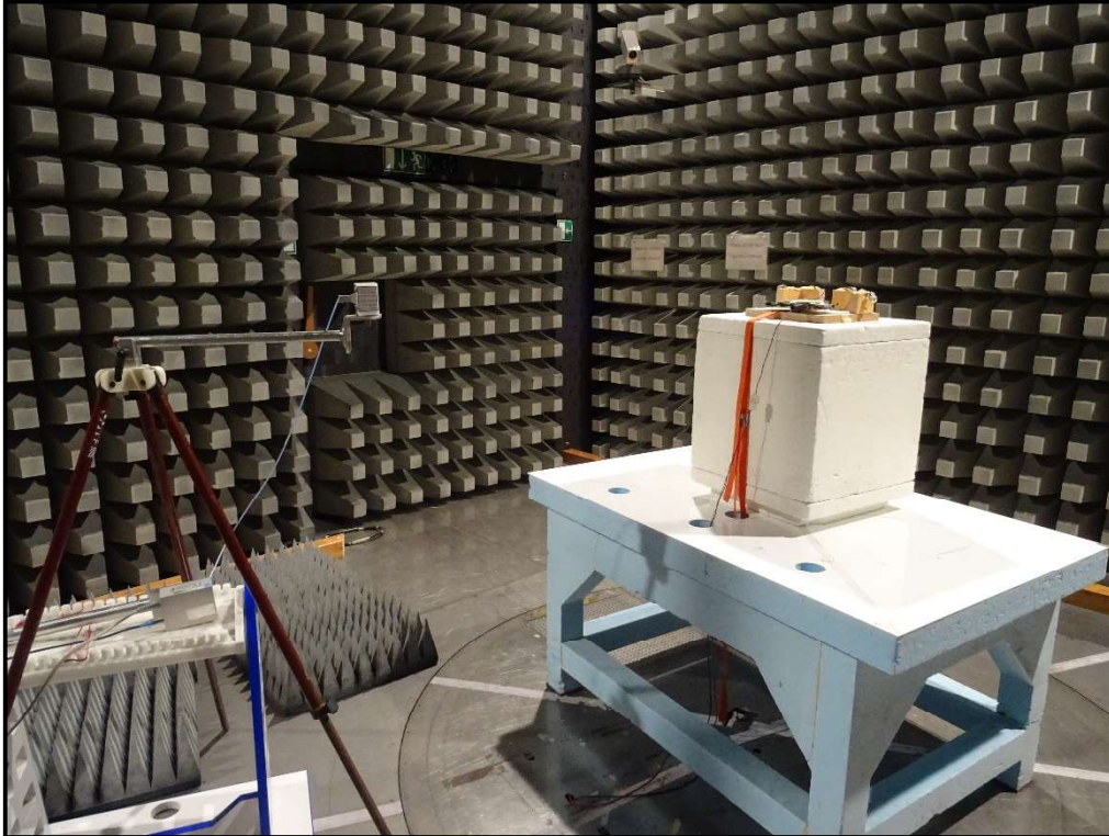
Photo 8: Terminated Ports 1+2+3+4 with 50 \Omega
