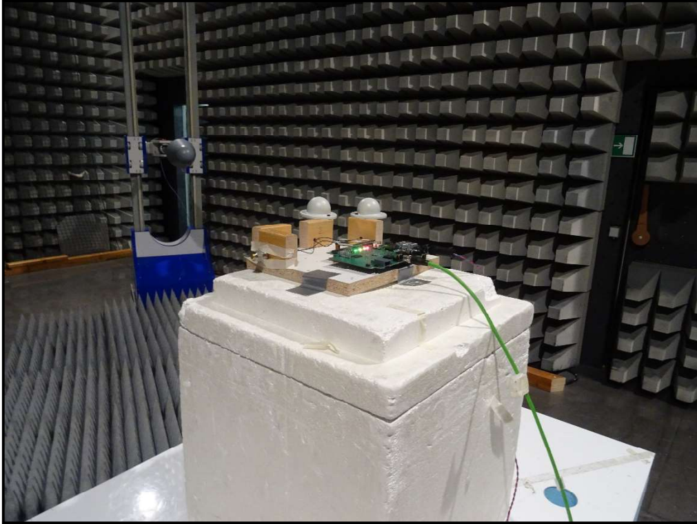
Photo 17: EUT- MIMO PORT 1+2 (Ports 3 & 4 Terminated with 50 \Omega )
