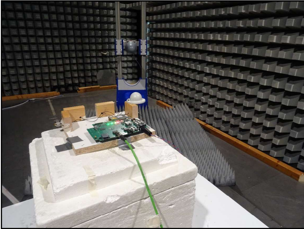
Photo 13: EUT- SISO PORT 1 (Ports 2,3 & 4 Terminated with 50 \Omega )
