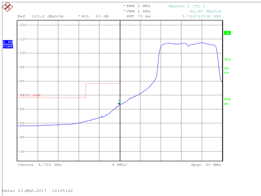
Figure 103 - Authorised Band Edge at 5725 MHz - Widest Emission Bandwidth
