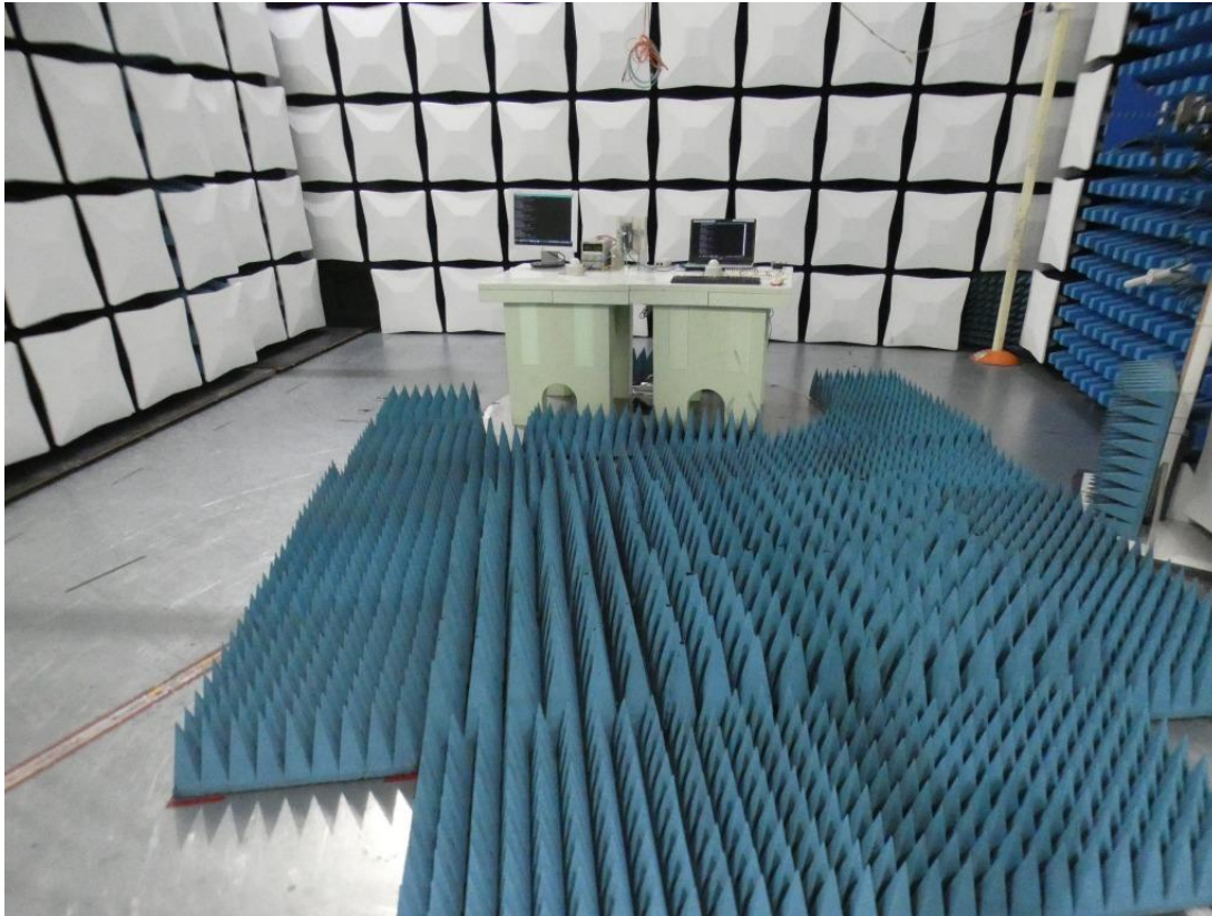
Photo 5: Test setup for radiated emissions measurements in semi-anechoic chamber with floor absorbers, (1 GHz to 18 GHz), front side view, computer peripheral setup
