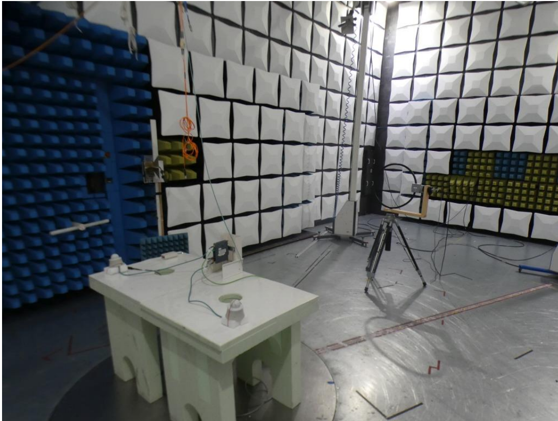
Photo 6: Test setup for radiated emissions measurements in semi-anechoic chamber (9 kHz to 30 MHz), rear side view
