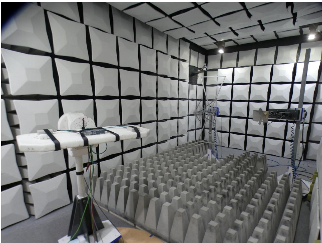
Photo 9: Test setup for radiated emissions measurements in fully -anechoic chamber (1 GHz to 26 GHz), right side view
