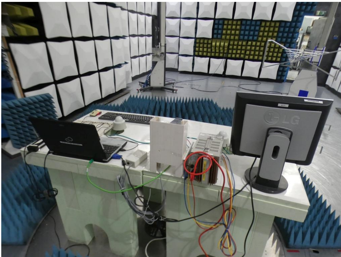
Photo 5: Test setup for radiated emissions measurements in semi-anechoic chamber with floor absorbers, (1 GHz to 18 GHz), rear side view [computer peripheral setup]
