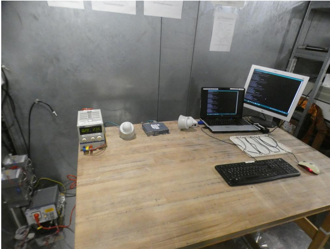
Photo 1: Test setup for conducted emissions measurements at AC Port, computer peripheral setup
