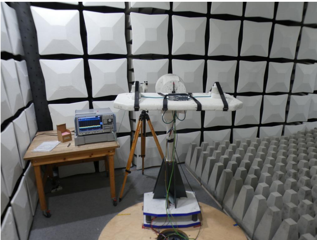
Photo 11: Test setup for radiated emissions measurements in fully-anechoic chamber (26 GHz to 40 GHz), right side view
