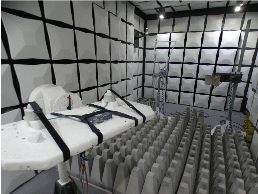
Photo 8: Test setup for radiated emissions measurements in fully -anechoic chamber (1 GHz to 26 GHz), right side view
