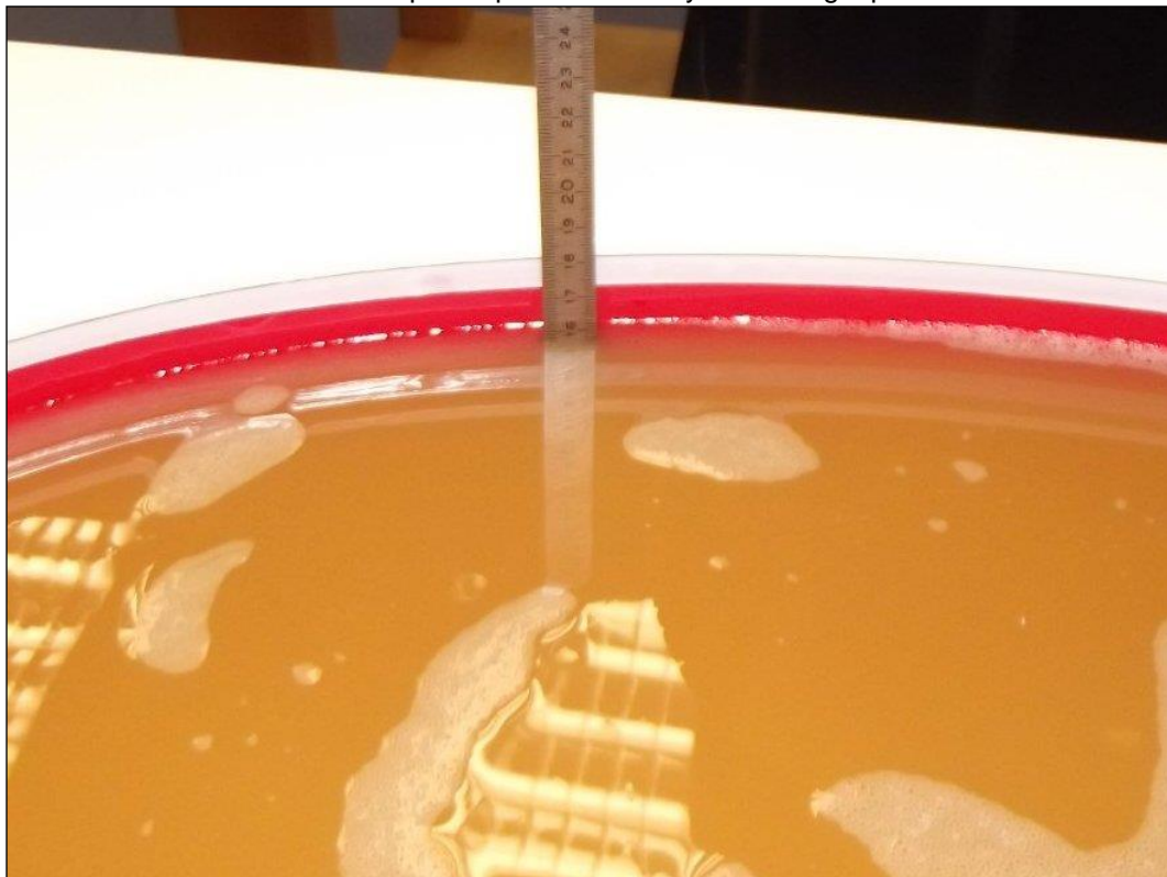
Photo 2: Liquid depth 5 GHz body simulating liquid
