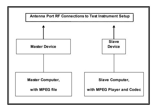
The EUT (Slave Device) does not have a display. All of the DFS software and driver software documented below in "Description of EUT" resides in the EUT. The Slave computer provides the streaming video player software and display capabilities for test purposes.
