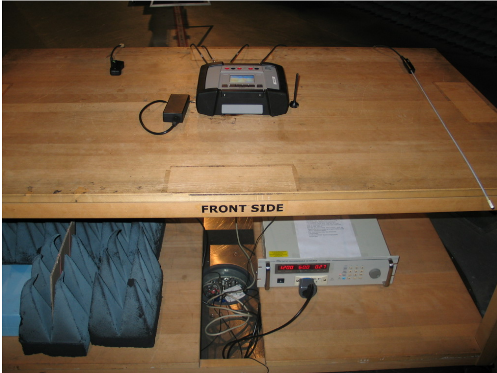
Photo 1: Test setup for radiated measurement
