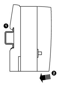
Follow the steps below to fit the SCALANCE W760/W720 to a DIN rail:
