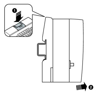
Follow the steps below to remove the SCALANCE W760/W720 from a DIN rail:
