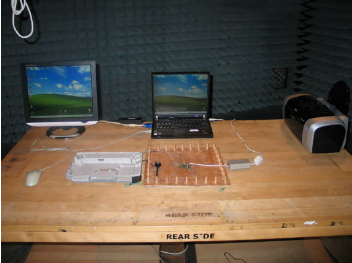
Photo 1: Test setup for radiated measurements
