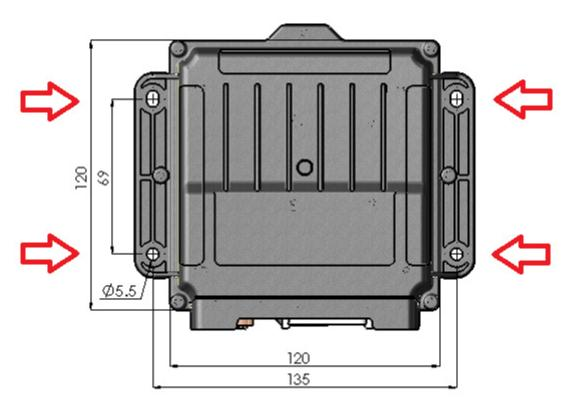
Fastening screws (M5 bolts) and washer are provided
