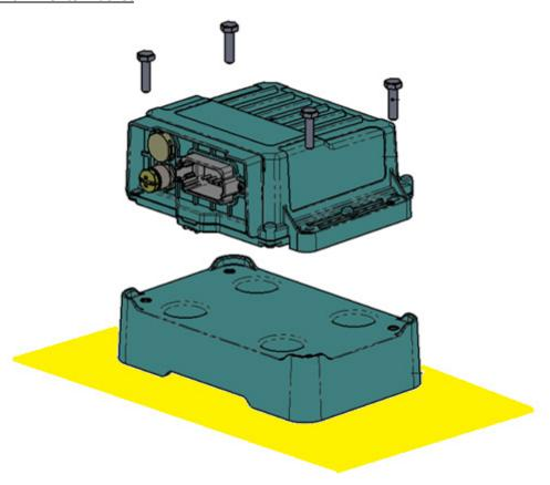
There are a total of 4 mounting screw holes, one at each corner, as pointed to by the red arrows below. Two of the holes are slightly elongated for tolerance purpose.
