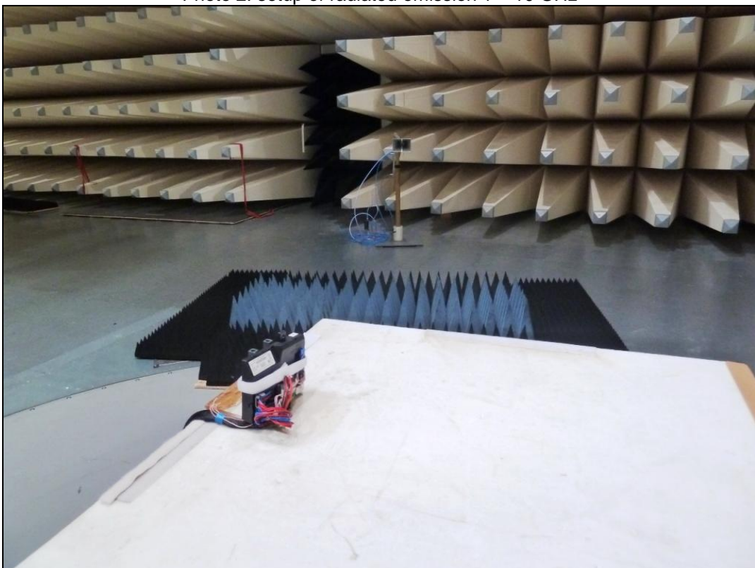
Photo 2: setup of radiated emission 1 – 10 GHz
