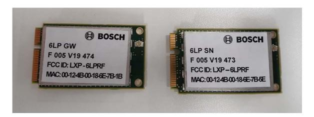
The label is a plastic material affixed using a permanent adhesive. (It is the same we use for automotive body computers and survives the heat cycles, oil tests etc. required for automotive)
