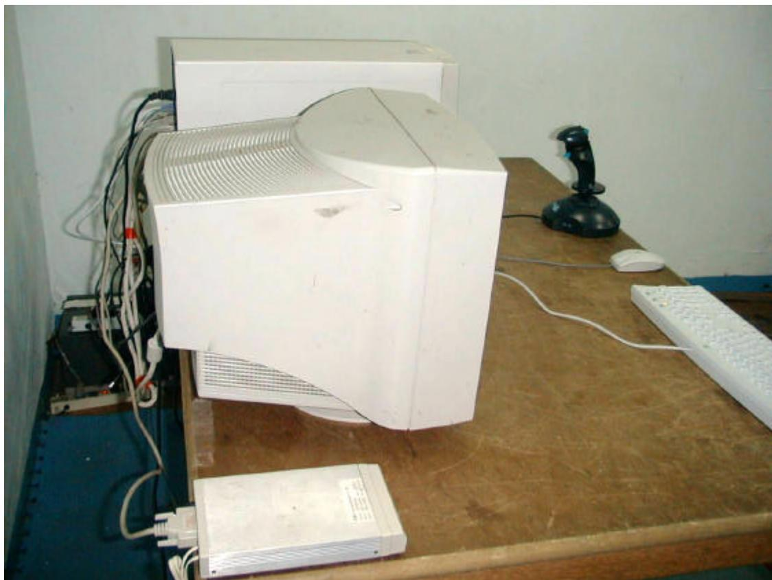
**Conducted Test Placement: (Photographs)(Test mode: USB by I.T.E.)**
