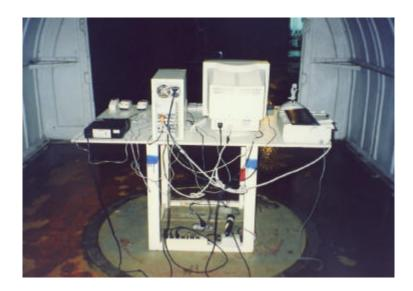
Radiated Emission Setup Photos (Worst Emission Position)
