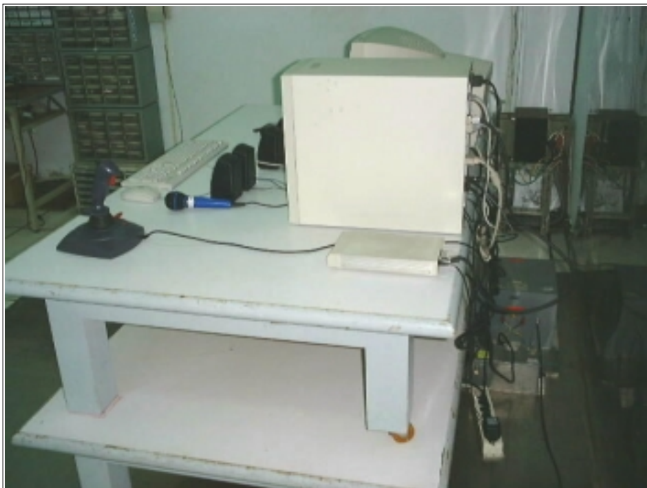
Conducted Emission Setup Photos (Worst Emission Position)
