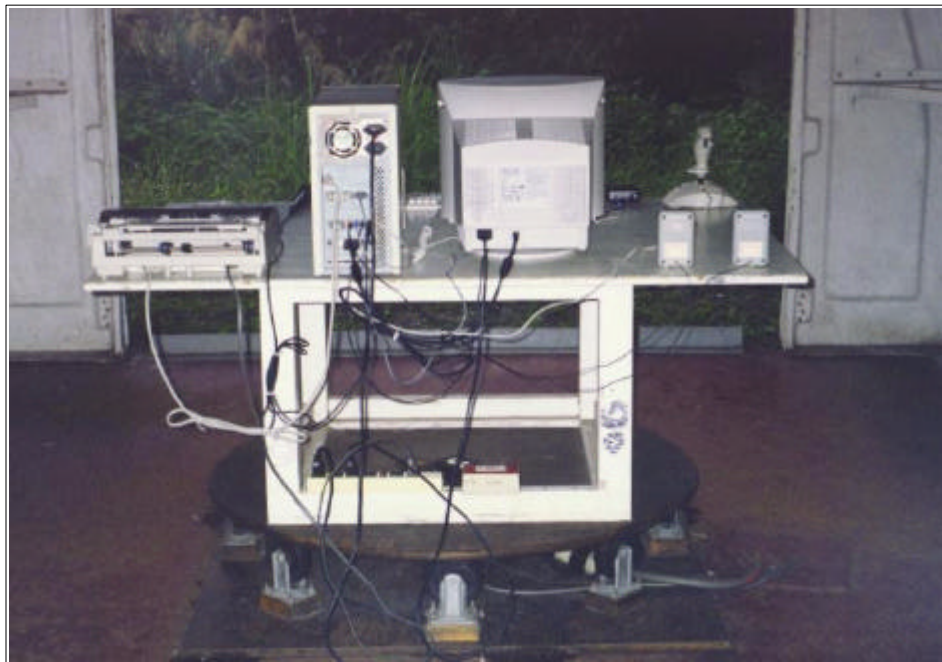
Radiated Emission Setup Photos (Worst Emission Position)
