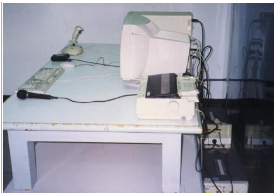
Conducted Emission Setup Photos (Worst Emission Position)
