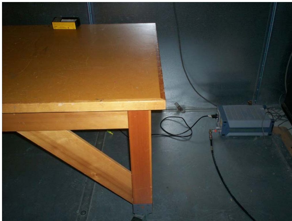
Figure 20 - Conducted Emissions Test Setup
