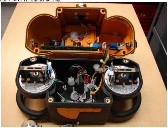
2. Transmitter/Coder board mounting.
