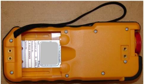
Please note that the Ergo F Transmitter will be packaged with the Battery Case not inserted on the battery compartment. This is to make sure that the label that shows the Transmitter's information (including FCC ID, IC ID, Model Name, Type, Frequency, Production No. and/or System No.) is clearly visible to the customer.
