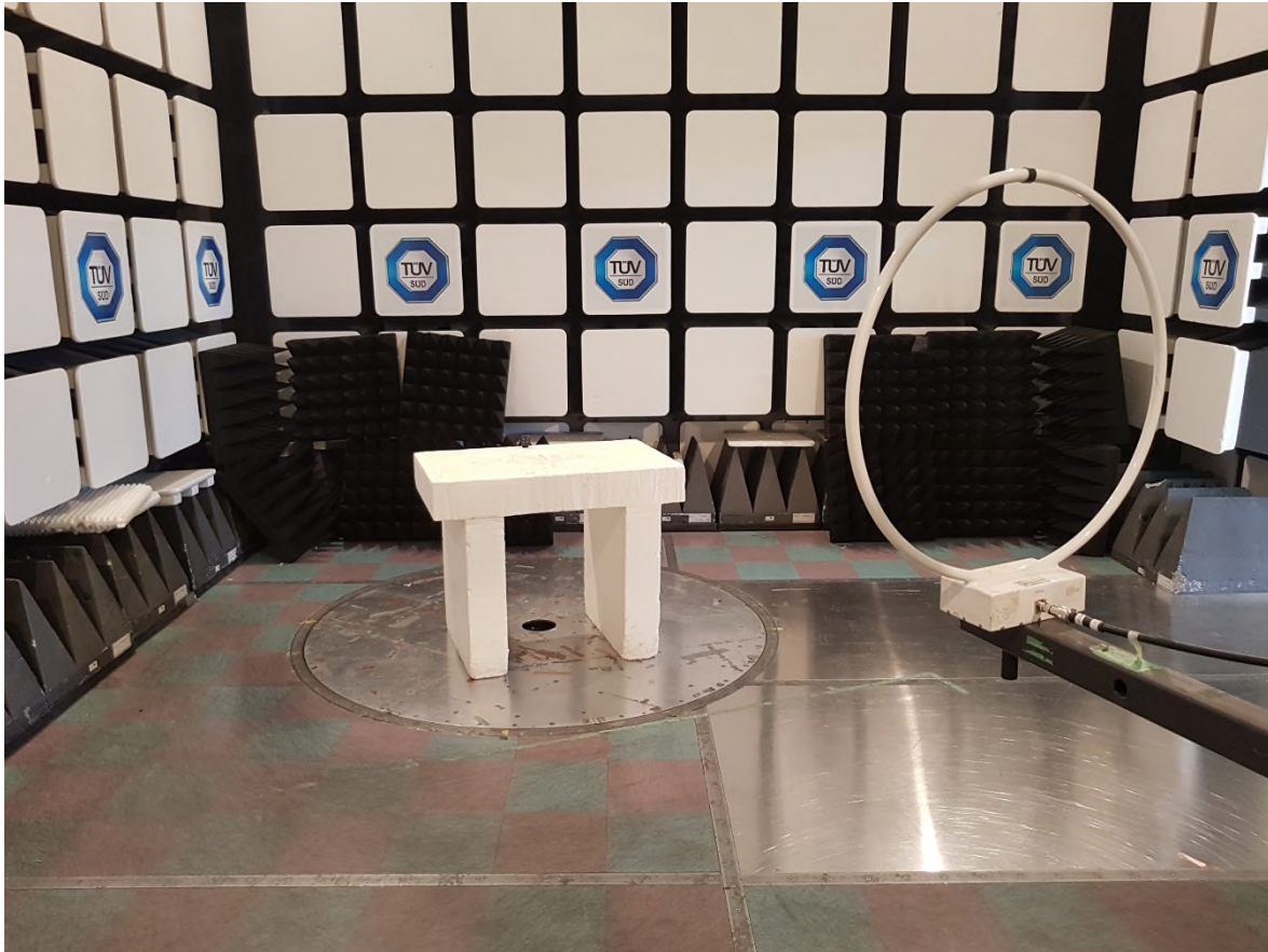
Figure 3 – Radiated Emissions Setup 9kHz – 30MHz
