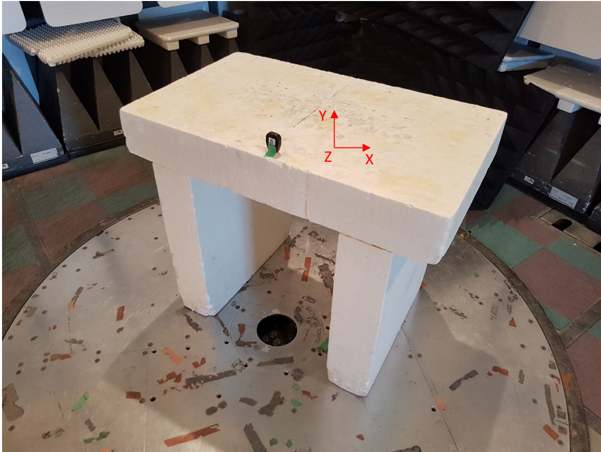
Figure 2 – Radiated Emissions Setup EUT in Y-Axis Position
