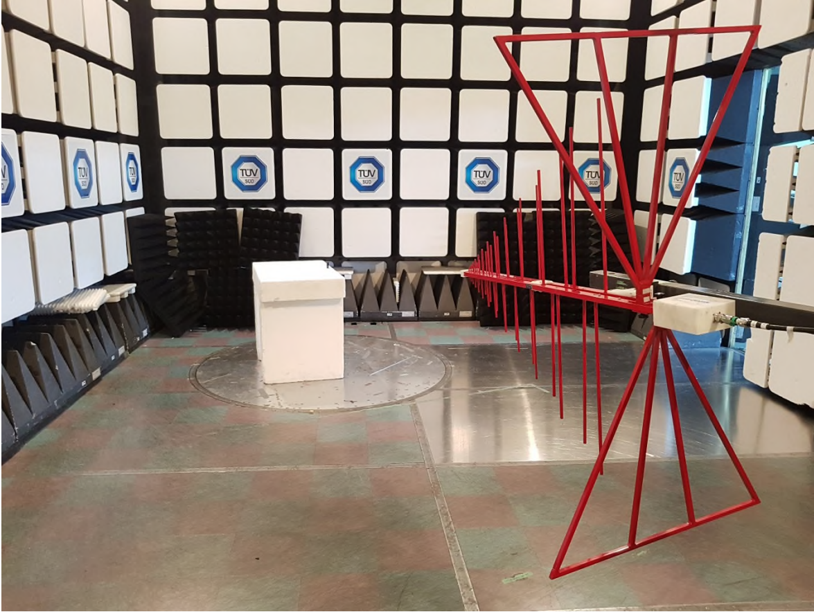
Figure 4 – Radiated Emissions Setup 30MHz – 1GHz
