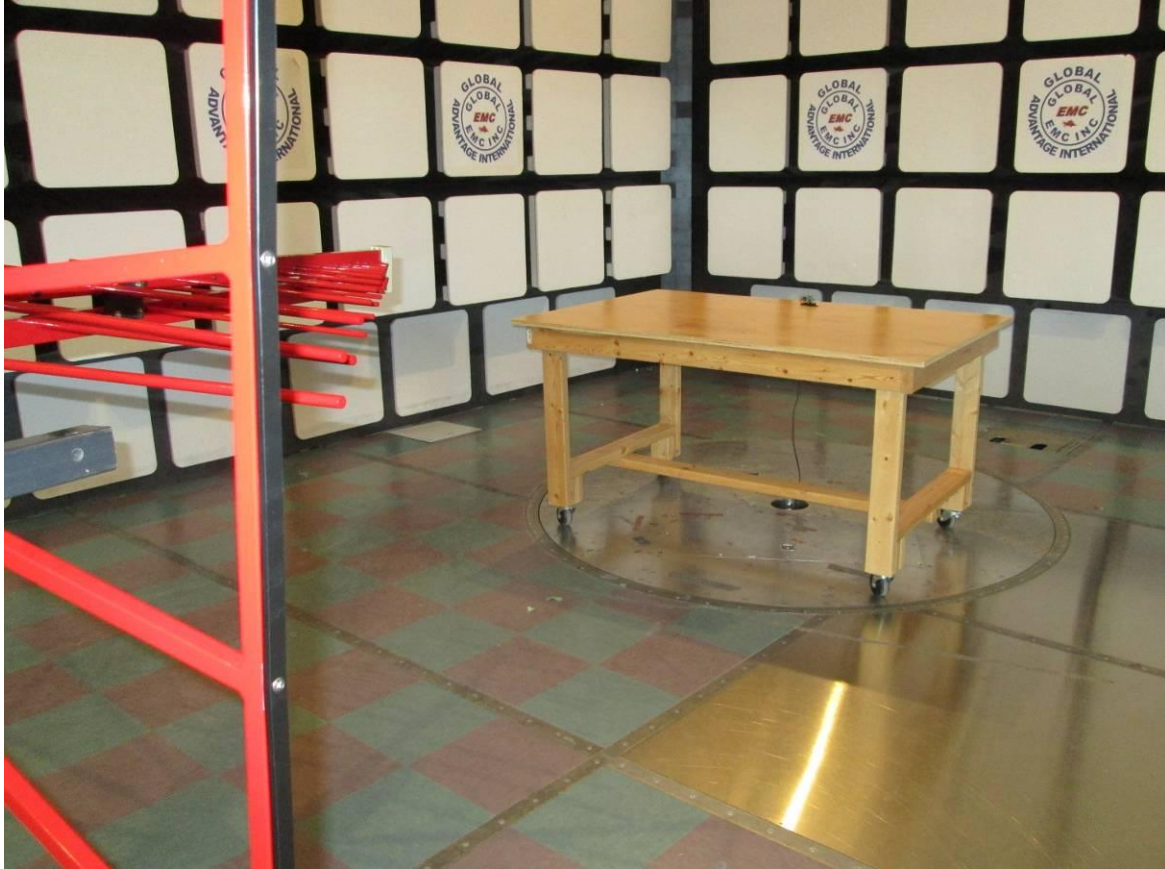
Radiated emissions testing (greater than 30MHz)
