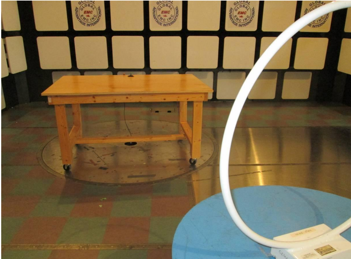
Radiated emissions testing (less than 30MHz)
