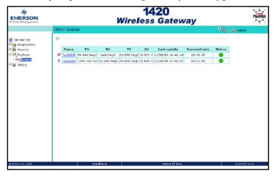
This page will display the transmitter's tag, PV, SV, TV, QV, Last Update, Update Rate, Battery Voltage, and Status. A green status indicator means that the device is working properly. A red indicator means that there is a problem with either the device or its communication path. For more detail on a specific device, click on the tag name.
