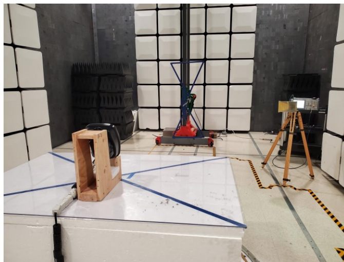
Figure 4 - Radiated emissions, 30 – 1000 MHz, rear
