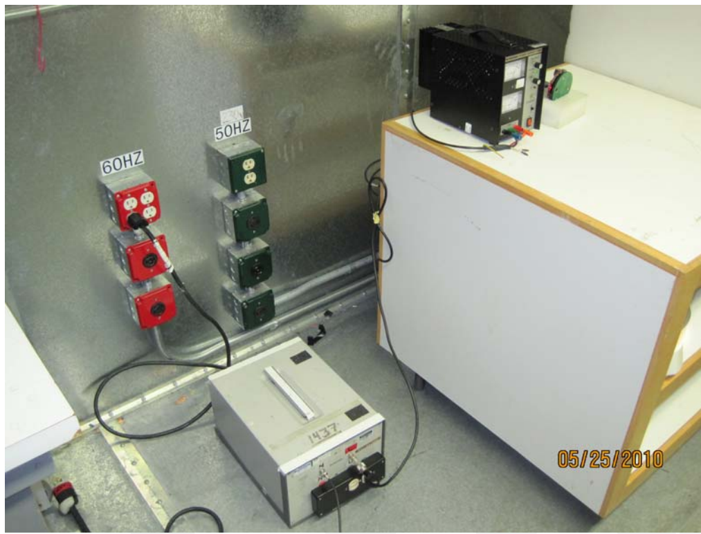
Test-setup photo(s): Conducted Emissions, AC lines, 150 kHz - 30 MHz
