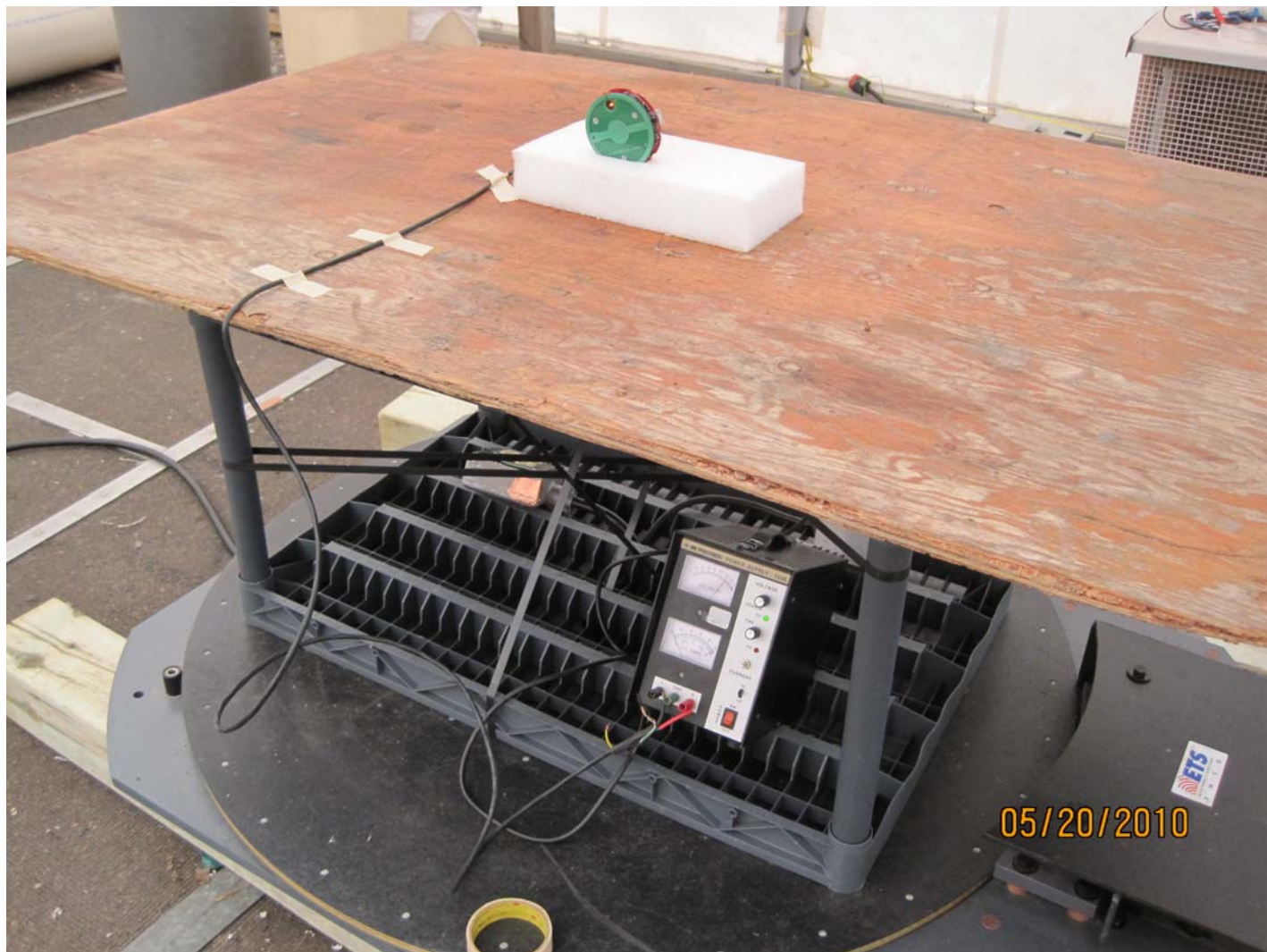
Test-setup photo(s): Radiated Emissions 30 - 1000 MHz
