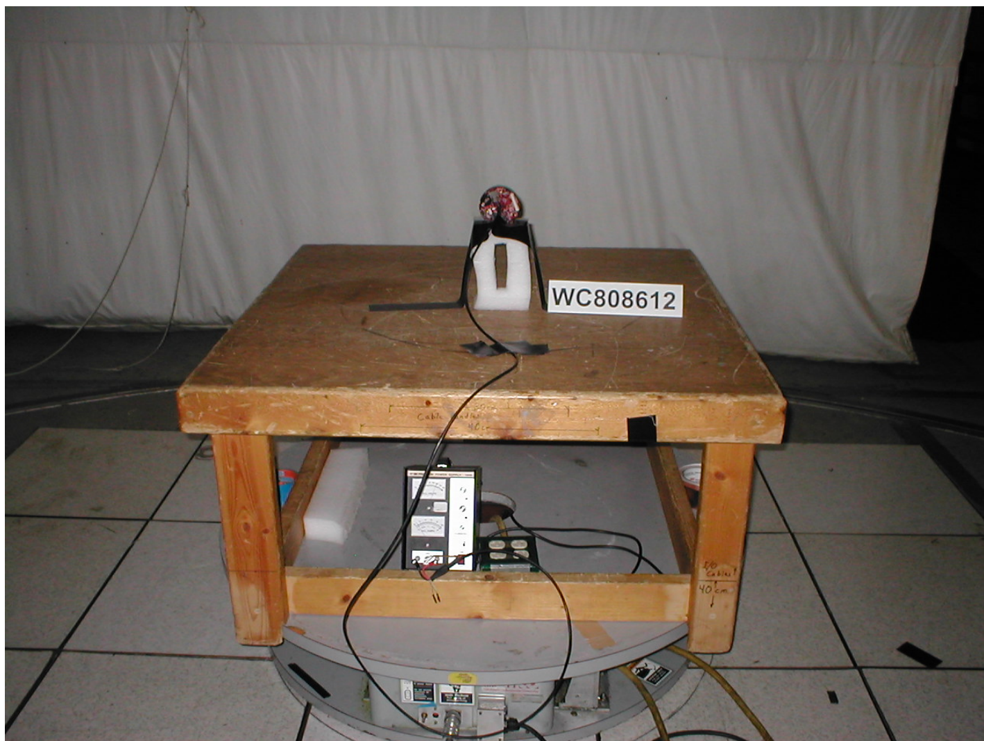
Test-setup photo(s): Radiated Emissions 30 - 1000 MHz
