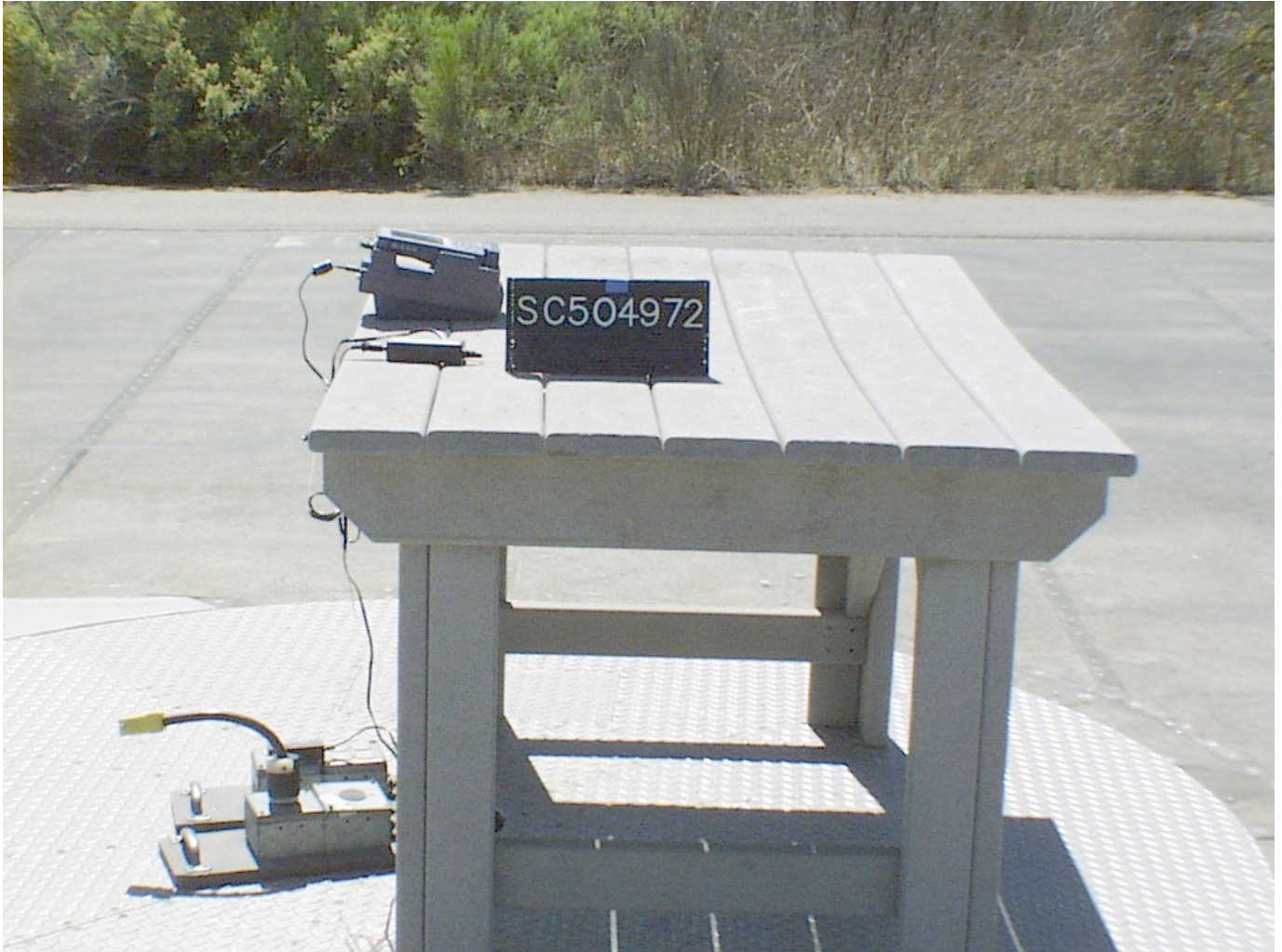
Photograph of Test Setup: Radiated Emissions
