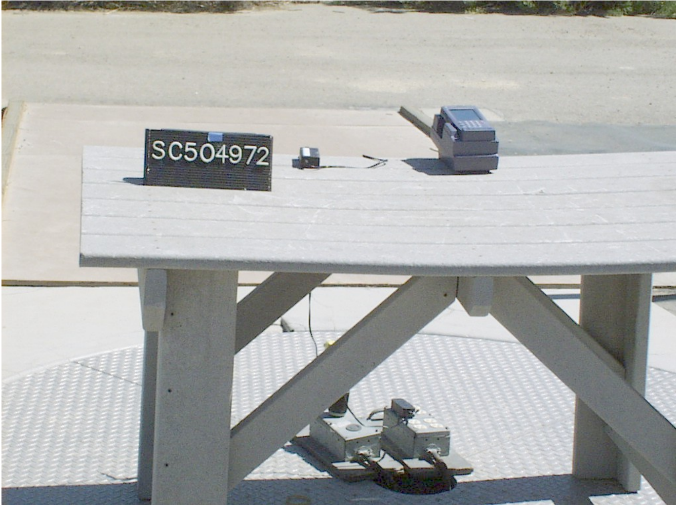
Photograph of Test Setup: Radiated Emissions
