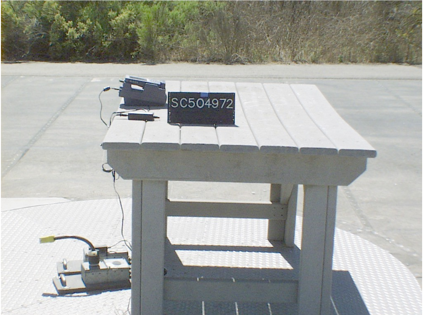
Photograph of Test Setup: Radiated Emissions
