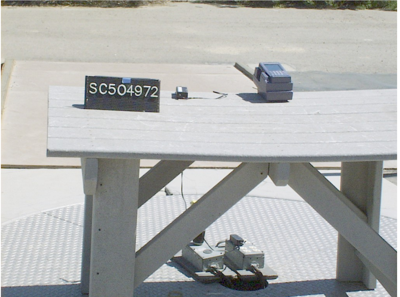
Photograph of Test Setup: Radiated Emissions
