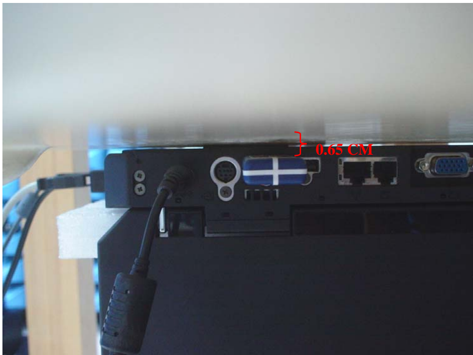
Fig.8 Photograph of the Bottom of the Pc is paralleled and at a distance of 0.0 cm from the base of the phantom, but 0.65 cm Spacing between EUT & Planar Phantom.
