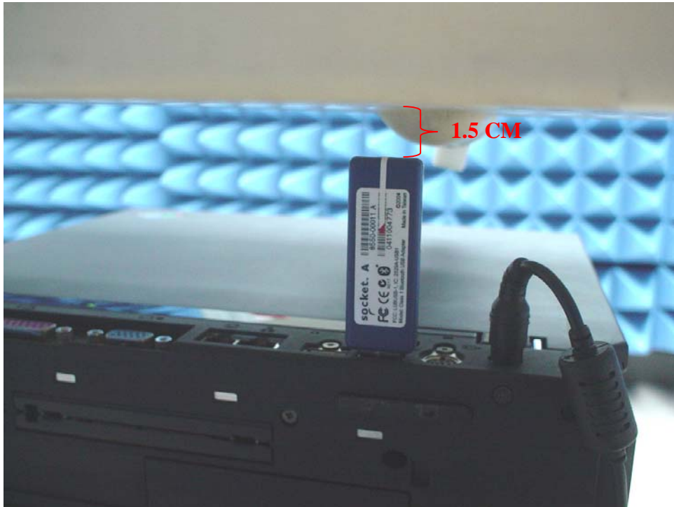
Fig.5 Photograph of the antenna tip is upward and at a distance of 1.5 cm from the base of the phantom.
