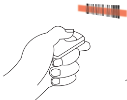
SocketScan S800 ~4" to 8" scanning distance
