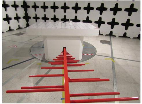
Radiated spurious emissions Test Setup Photo-Horn Antenna
