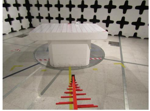
Radiated spurious emissions Test Setup Photo-Horn Antenna
