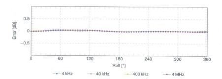
SPEAG axial deviation from the ideal response tolerance for E-field:  $\pm 0.8\,\mathrm{dB}$
