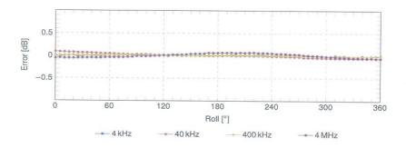
SPEAG axial deviation from the ideal response tolerance for H-field:  $\pm 0.6\,\text{dB}$
