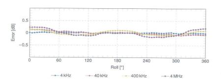
H-Field Receiving Pattern ( $\phi$ ),  $\vartheta = 90^{\circ}$
