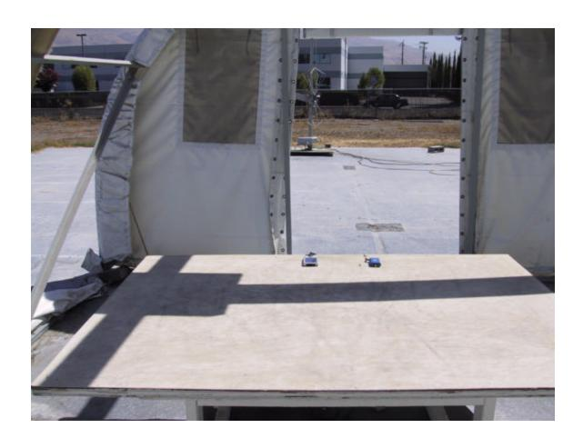
**Photograph 1. Radiated Emissions Test Setup (Front View)**
