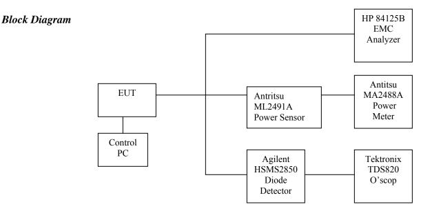
The solid lines are coaxial cables and the dashed lines are either EUT insertion to the test board or control cables between test setup devices. The measurement results were adjusted with the attenuation of the coaxial cable.
