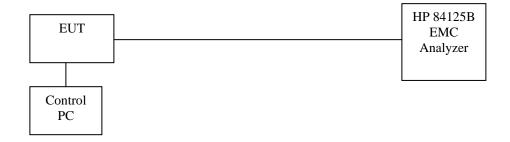
The solid lines are coaxial cables and the dashed lines are either EUT insertion to the test board or control cables between test setup devices. The measurement results were adjusted with the attenuation of the coaxial cable.
