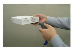
When data is read and sent to device, the scanner beam will turn off. Depending on your settings, the scanner may beep and/or the CHS's LED may flash green to indicate a good read.
