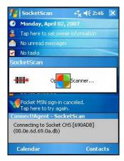
5. After the devices connect, the CHS will beep once. The SocketScan icon at the bottom of the Today screen will change into a scanner icon to indicate the connection.
