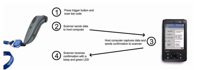
The most likely source of errors in any cordless scanning system is not in the scanning and decoding process, but in the transmission of the data to the host. For this reason, the Cordless Hand Scanner features the exclusive *Error Proof Protocol* (patent pending) from Socket Mobile, which ensures that scanned data is
