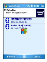
To help you identify the scanner, Connect! Agent reports the scanner's Bluetooth MAC address. The last six characters are displayed after the Bluetooth device name.
