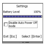
By default, the CHS will automatically turn off when there is no *Bluetooth* connection in 20 minutes. If desired, check **Disable Auto Power Off mode** if you would like the CHS to always stay on. Press the **Enter** button on the right side.
