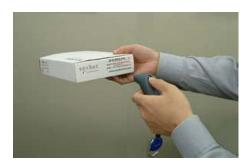
When data is read and transmitted to the host, the scanner beam will turn off. Depending on the settings chosen in the SocketScan Configure screen, the scanner may beep and/or the LED may flash green.
