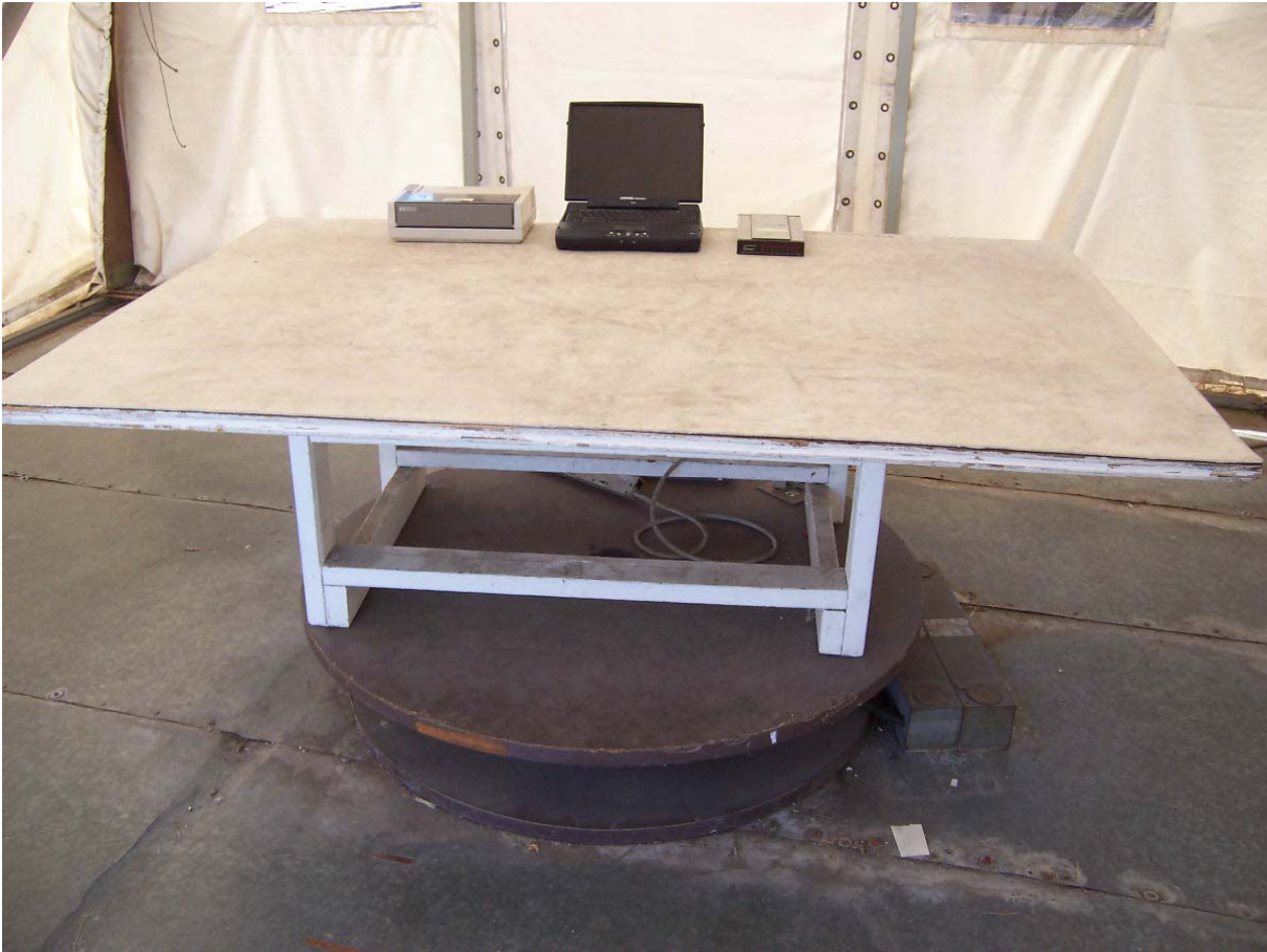
Radiated Emissions Test Setup
