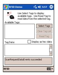
3. Hold the device in the correct position to read an RFID tag, as described in Chapter 2. Hold the device so the SOMO 655 RFID Reader Card is <u>parallel</u> to and directly above the tag, at most 2.0 inches above the tag.
