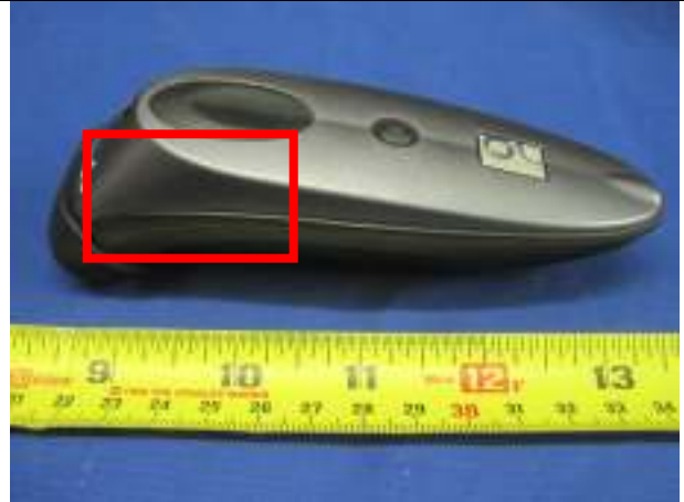
Left Edge position against flat phantom (separation distance – 0cm)
