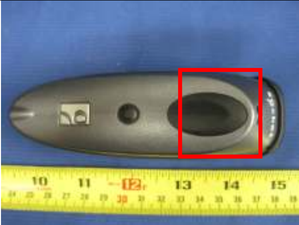
Top position against flat phantom (separation distance – 0cm)
