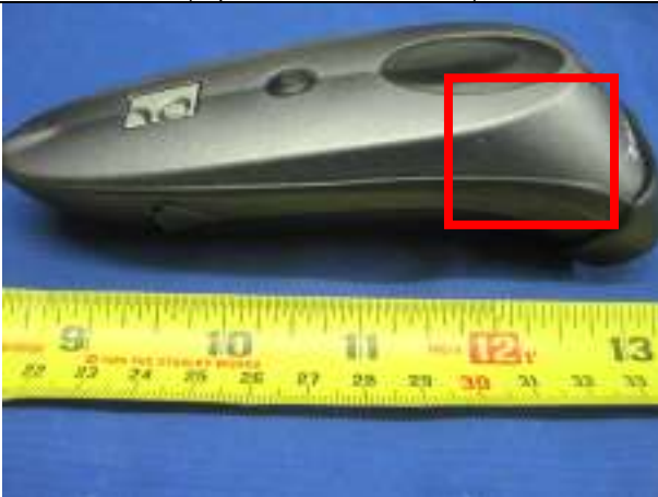
Right Edge position against flat phantom (separation distance – 0cm)
