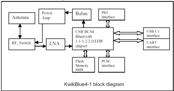
From the diagram, the Power Amplifier provide 20dBm gain for the Bluetooth TX\_power. This make this module into a class-1 bluetooth module.
