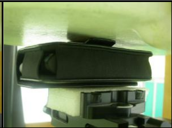
The bottom of the EUT face to the phantom with 0mm-separation distance.
