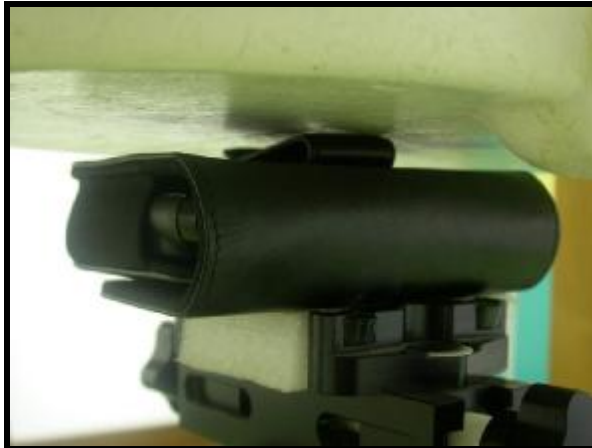
The front of the EUT face to the phantom with 0mm-separation distance.
